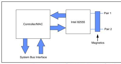
Figure 1. 82555 10/100 Mbps Ethernet Solution
